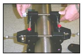
Figure 3-9: Installing Nuts onto the Fixture
